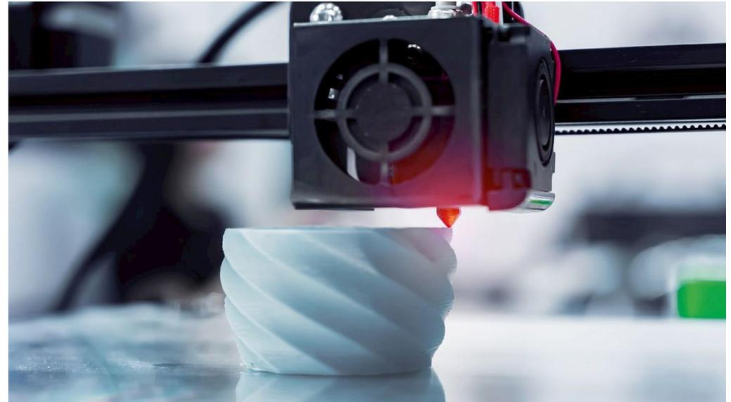
*Additive manufacturing is the process of printing multiple, stacked layers of material to create finished products with complex geometries. The parts can be used for aerospace, automotive, and industrial applications!*
