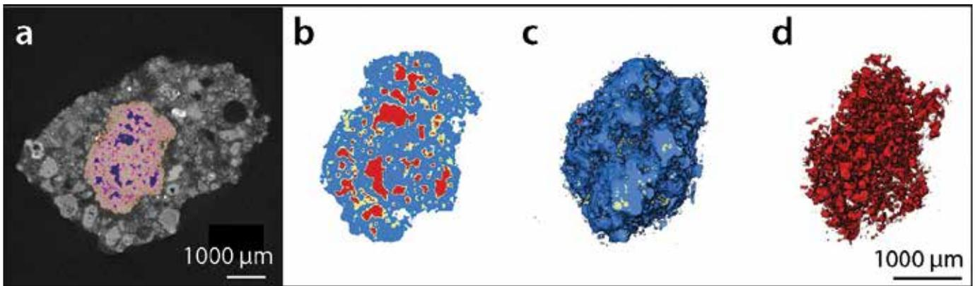
**Figure 3.** a) X-ray tomography of a sample of Trajan's Markets mortar, with Pozzolane Rosse scoria highlighted. b–d) 3-D segmentation of scoria shows residual glass (blue), cementitious hydrates (yellow), and pore space (red).
