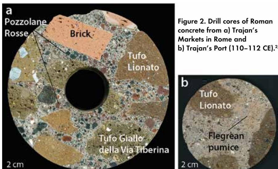
**Figure 2. Drill cores of Roman concrete from a) Trajan's Markets in Rome and b) Trajan's Port (110–112 CE).<sup>2,3</sup>**
