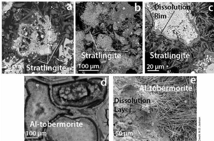
**Figure 4.** Mineral cements in ancient mortar samples. Strätlingite crystals in (a) Caecilia Metella mortar, (b) 180-day mortar reproduction sample (Figure 5), and (c) Trajan's Markets mortar. Al-tobermorite in (d) Baianus Sinus pumice sample and (e) Surtsey basalt from 2017 SE-02B core at 120°C and from 107.5 m-below surface.
