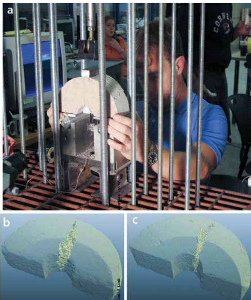
**Figure 5.** Analysis of reproduction of Trajan's Markets mortar. a) P. Brune performing a fracture testing experiment. X-ray tomography results for fractures at (b) 28 days or (c) 180 days of hydration.
